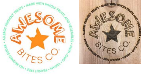
Figure 1: Awesome Bites CO into a piece of wood. This particular engraving took a total time of 1 hour and 43 mins at 500mm/min with a 2000 mm/min velocity override. This image had an area of 125x125 mm
