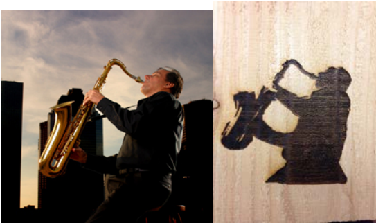
Figure 2: Here in our second image we engraved an image of Dr. Trombetta playing a saxophone. This engraving took a total time of 1 hour and 16 mins at 500mm/min No velocity override 75x75 mm
