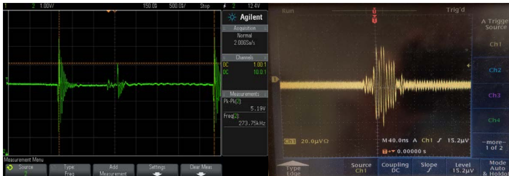
Figure 1: Oscilloscope traces for before (5.19 Vpp) and after (96 \mu Vpp) filtering.
