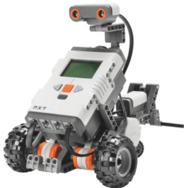
Figure 1. This is the NXT robot that will be used to perform the tests. The ability of this robot to detect a specific target will aid in the landing of a jet
