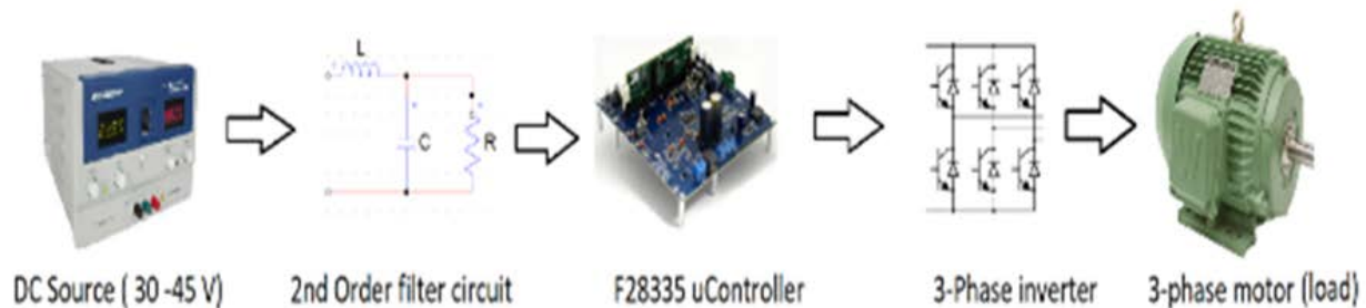
Fig. 1. Circuit Diagram of Filter and 3-Phase Inverter
