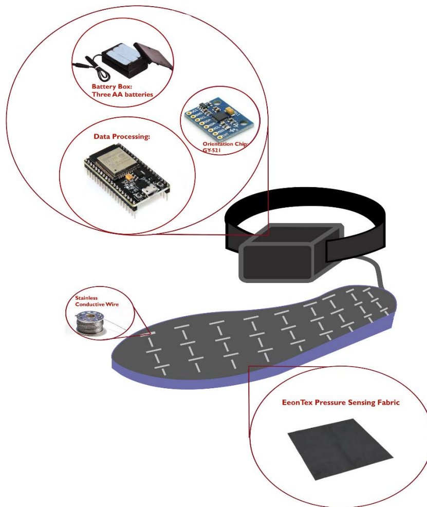
Fig 1. The black box houses all the internal electronic components used to gather and process data. The pressure sensor insole is composed of a fabric material and lined with conductive wiring to create variable resistive points at each intersection.
