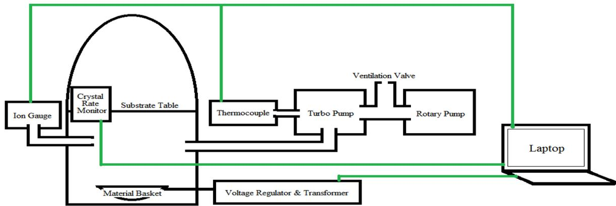
Figure 1: Thin Film Thermal Evaporator Schematic
