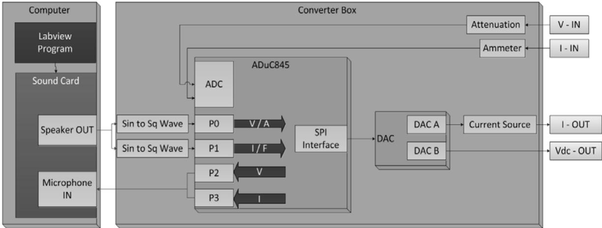
Figure 1 - Block Diagram for Source Meter
