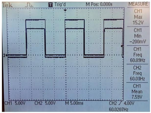
Figure 3. Oscilloscope image showing the output of the phase matching circuit. The output of the PLL (top) signal is matched with that of the grid signal (bottom).
