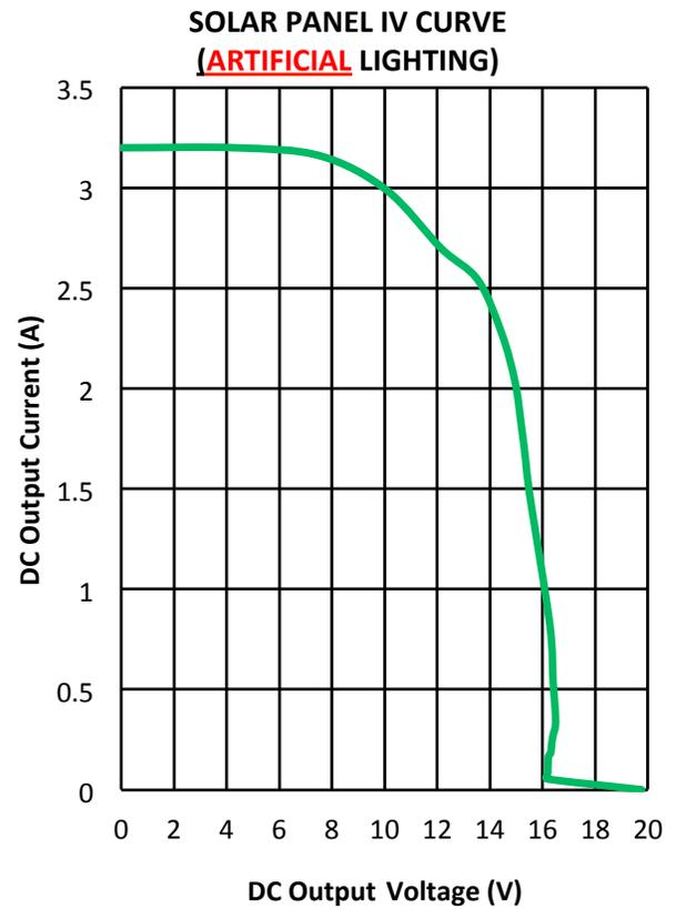
Figure 1. Solar panel IV curve under artificial lighting conditions.
