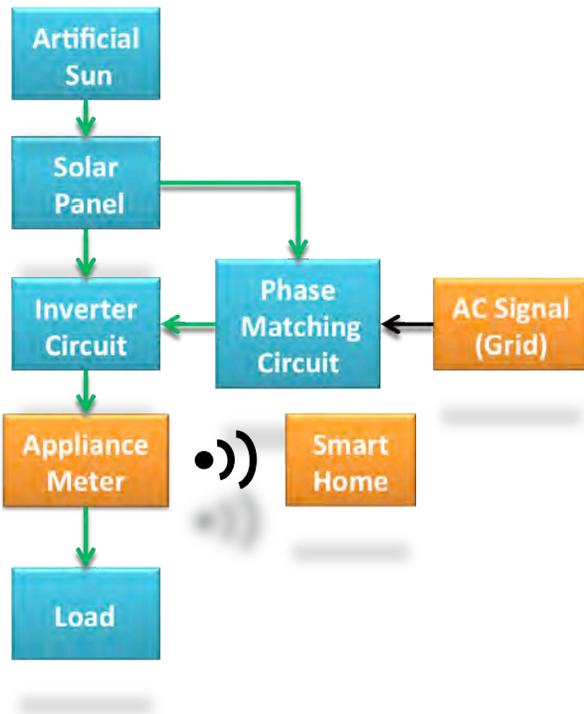
Figure 1. Overview diagram of the Solar Panel Interface to Smart Home.
