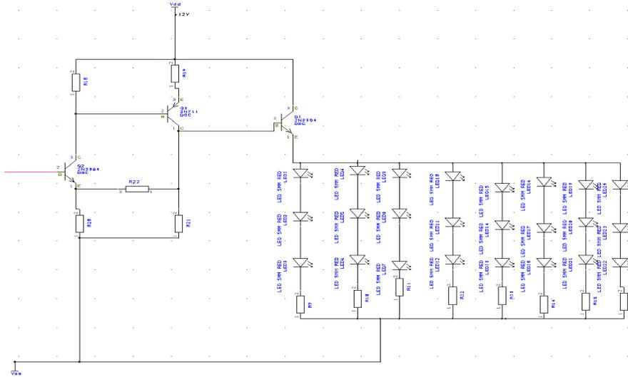
Figure 2 - LED Driving Current and Voltage Amplifier Schematic
