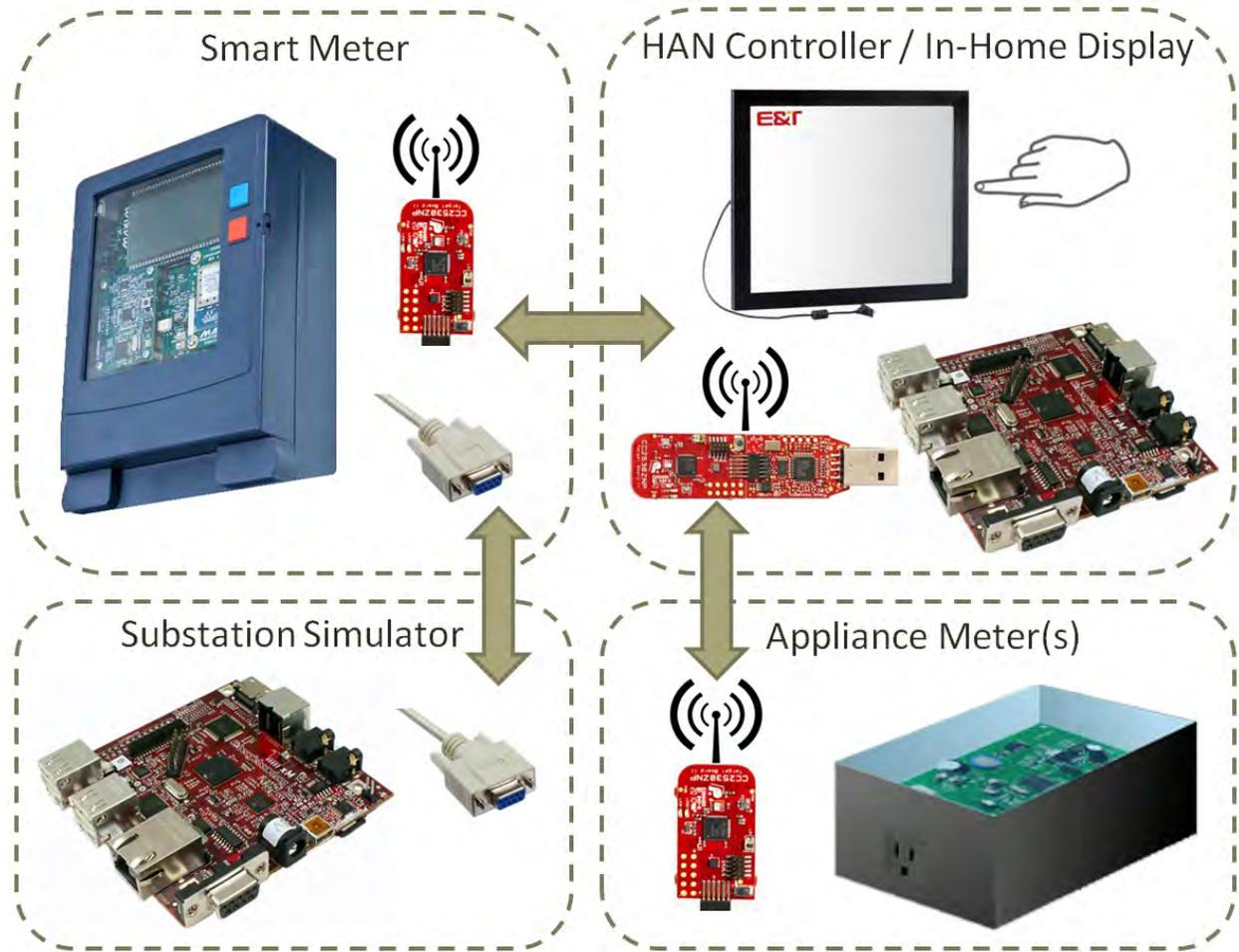
Figure 1 - Smart Home Energy Metering System
