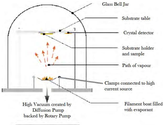
Figure 2: Bell Jar Thermal Evaporator Chamber. Credit: <http://www.betelco.com/sb/phd/ch3/c34.html>
