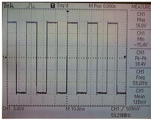
Figure 2. Oscilloscope image showing the output of the inverter circuit before stepping-up the voltage to 120 [V].
